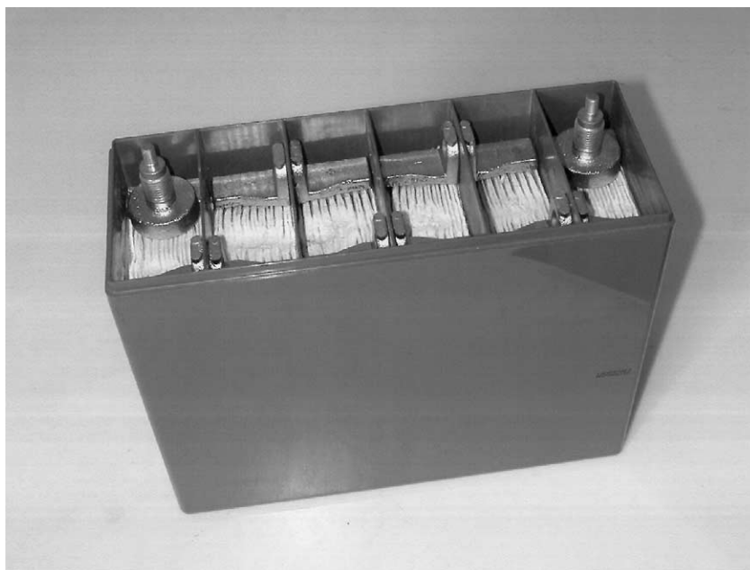
Fig. 2. A 12 V six cell monobloc with lid removed.
